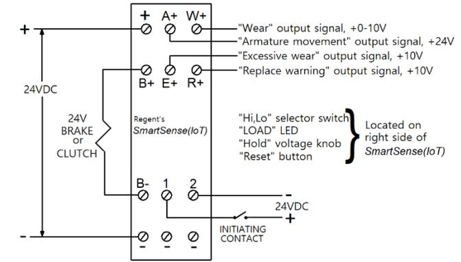
All "-" terminals are internally connected and are common reference for all output signals.
